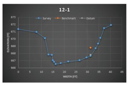
All of this data was used to create three graphs for each of the 15 locations. The first graph illustrates the x-section of the stream where the data logger was installed.
