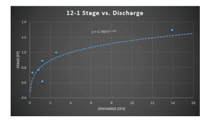
The third graph is the Stage vs. Discharge graph, which allows us to estimate the amount of flow in that section of the stream during various water levels (or during rain events). The blue dots are the actual field measurements taken by field crews.
