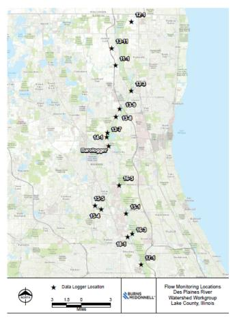
Field measurements were taken six times at the 15 locations to confirm that the data collected by the loggers reflected actual field conditions.
