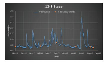
The second graph shows the elevation of water in the stream over time. The red dots are where the actual measurements were taken by field crews.
