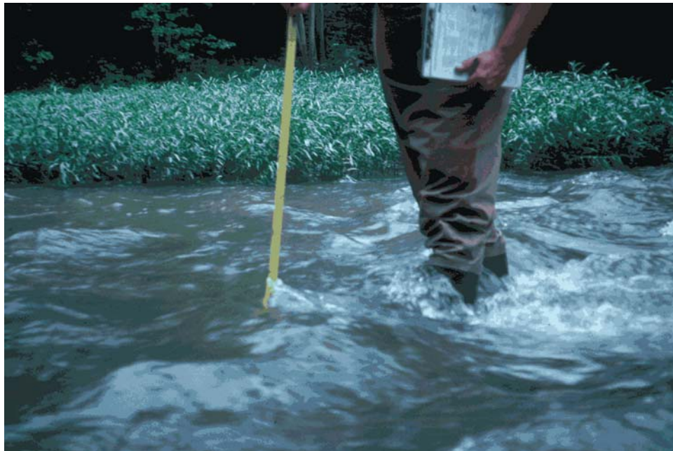
Estimating current velocity, Sharp drop from front to back of rod and boot indicates fast current velocities.
